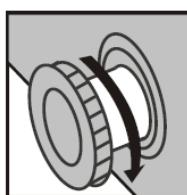
• Rotate the drain dial 180 degree. This will let the water flow out in the tray. When done, push the drain dial in. Re-plug the drain plug inside the freezer compartment. Note: monitor the container under the drain to avoid overflow.
