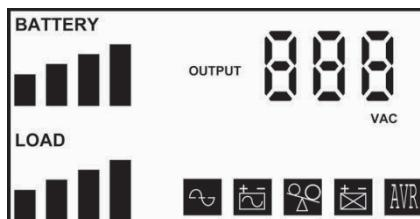
Battery: Battery capacity (25%, 50%, 75%, 100%)
