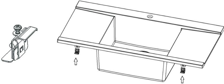
3.7. Carefully tighten the clips fastening the sink to the worktop.
