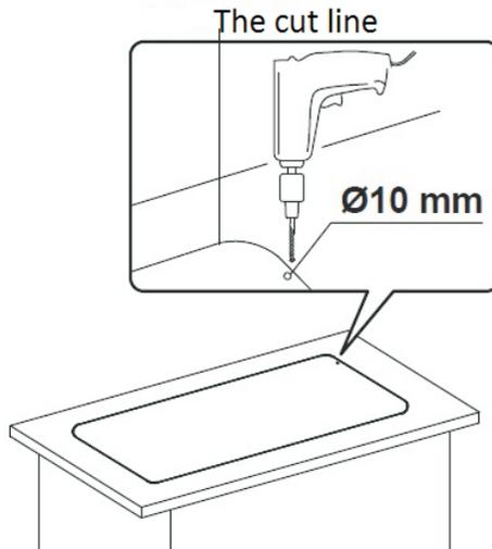
**3.3.** Using the jigsaw carefully cut along the cut-out hole.
