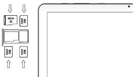
Attention! It is possible to use either two SIM cards (nanoSIM) or one SIM card and microSD card at the same time. Do not insert the memory card into the SIM card slot. If the memory card is stuck in the SIM card slot, contact the authorized Sigma mobile service center for safe removal. Be careful not to lose your SIM card and do not let others use it.
