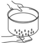
Dry the inner pot and confirm there are no impurities on the heater. Put the inner pot in the electric cooker and then turn the inner pot around to allow the pot to be in full contact with the heater. Don't fill water in the outer pot for avoidance of any failure or electric shock.
